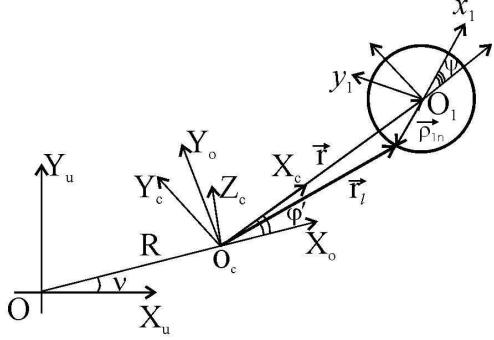
$$\ddot{r} = \dot{\bar{r}} + \dot{\phi} \bar{e}_r + \ddot{\phi} \bar{e}_{Y_c}, \quad \ddot{\bar{r}} = r \ddot{e}_r, \quad \ddot{r} = r \ddot{e}_r + r \dot{\phi} \bar{e}_{Y_c},$$
